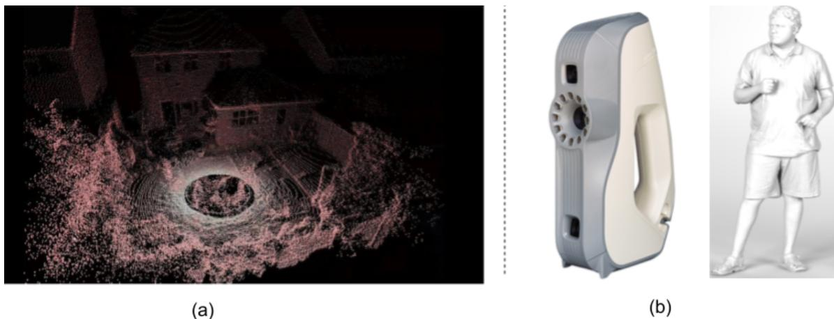
**Figure 1.4** a. Sample LIDAR scan of a house, Image adopted from cite b. Structured light Artec Eva sensor and a sample scan
