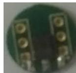
Figure 3-7: PCG Sensor Printed Circuit Board (10x10mm)
