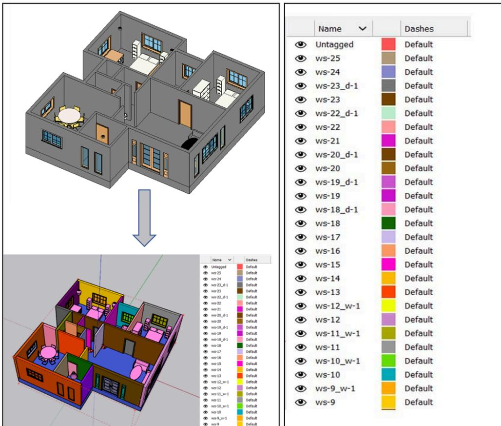
Figure 3.2. Flowchart for space model and IFC Conversion
