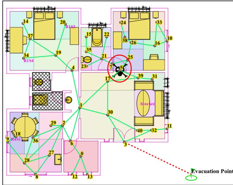
Figure 5.2. : Floor plan with blocked node.
