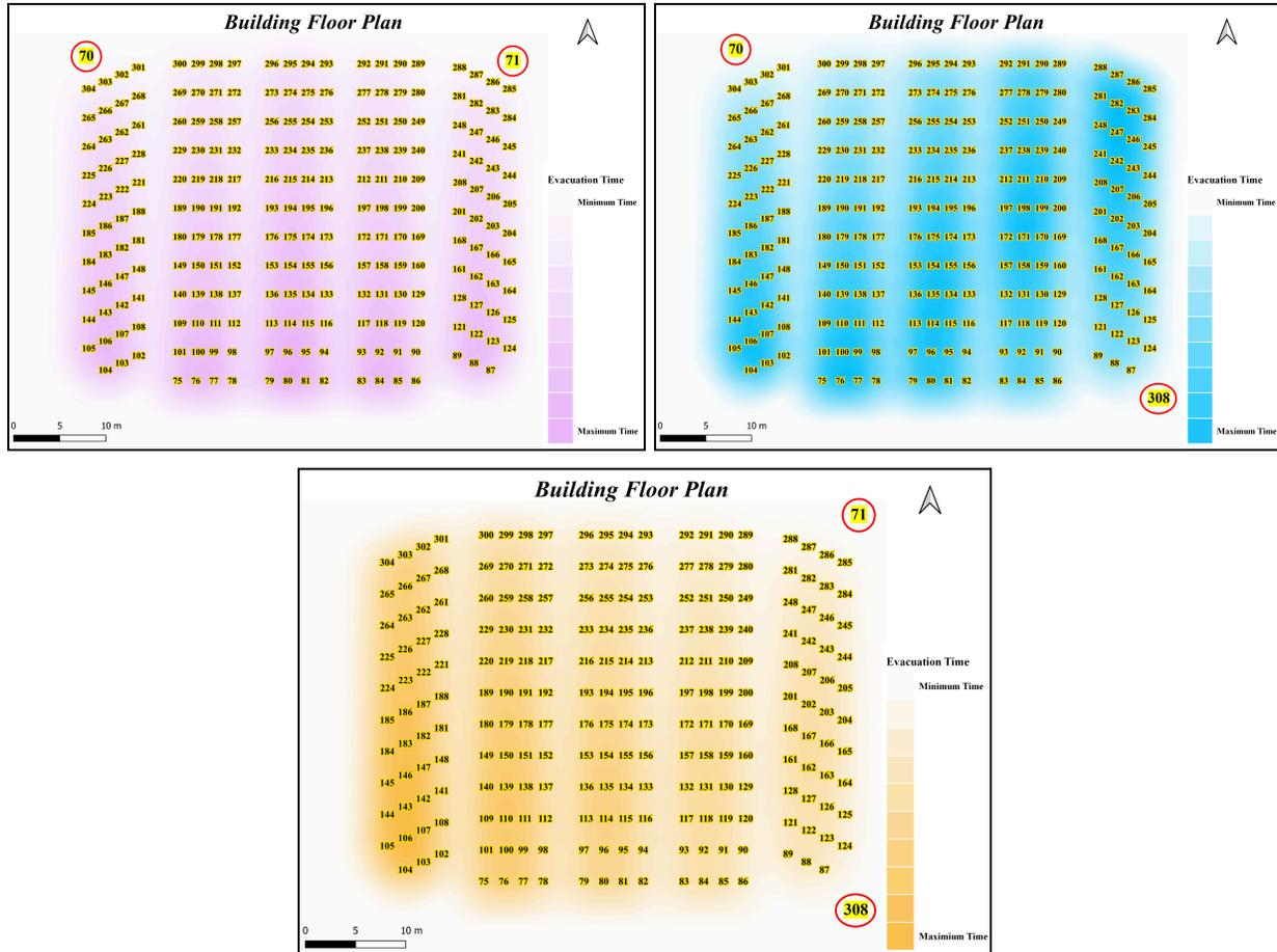
Figure 6.6. Building floor plan with maximum and minimum time through (a) door 70-71 (b) door 70-308 and (c) door 71-308
