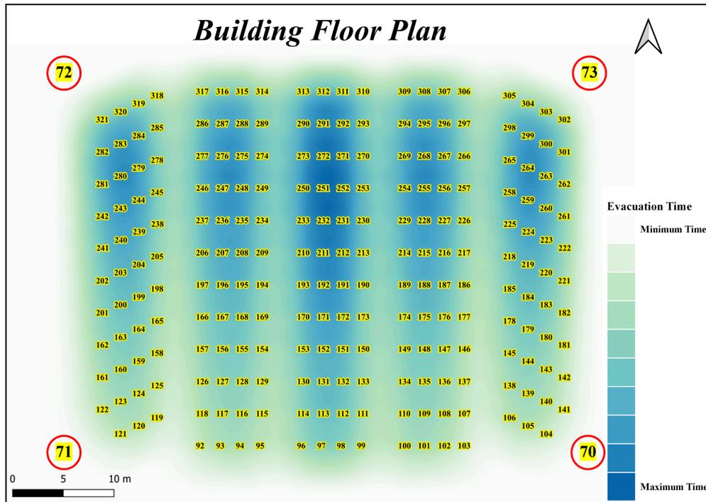
Figure 6.4. Building floor plan with maximum and minimum time through all the doors
