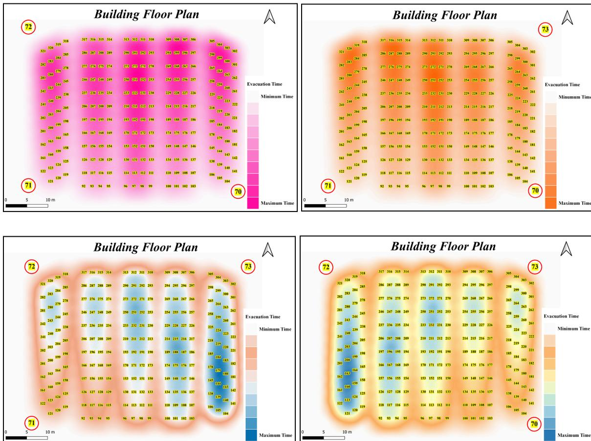
Figure 6.3. Building floor plan with maximum and minimum time through (a) door 70-71-72 (b) door 70-71-73 (c) door 72-71-73 and (d) door 73-72-70
