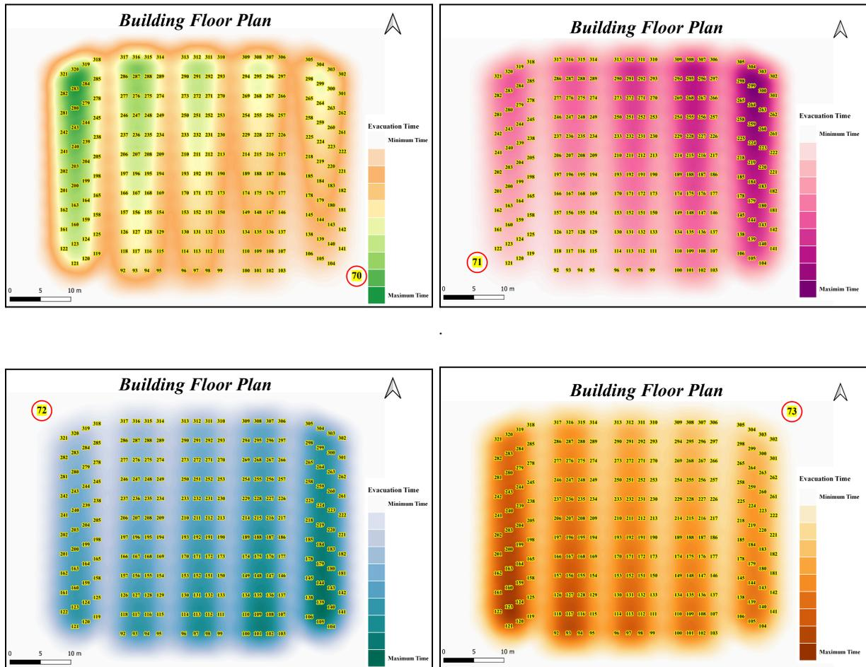
Figure 6.1. Building floor plan with maximum and minimum time through (a) Door 70 (b) Door 71 (c) Door 72 (d) door 73
