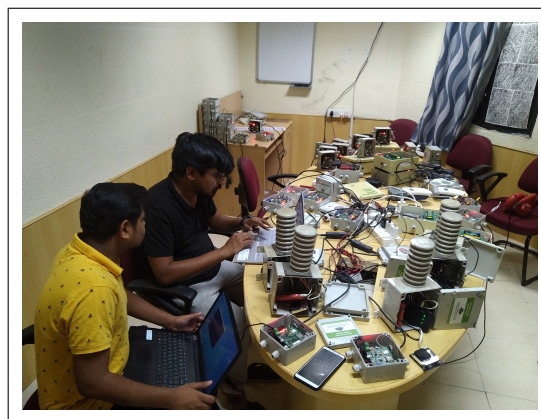
Figure 5.5: Ensuring accuracy through seasonal maintenance of dust sensors
