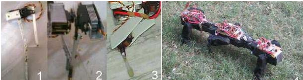
Fig 6.0 Leg design and the hexapod version
