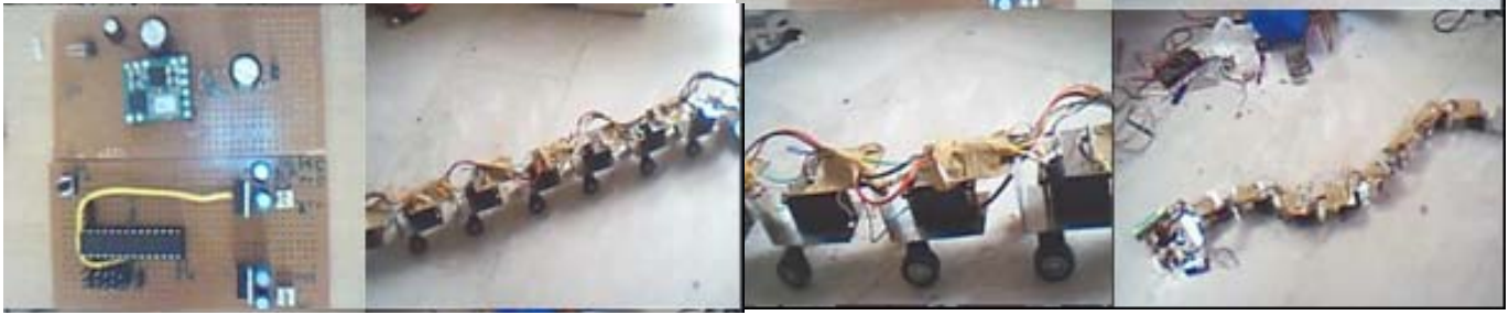
Fig 5.0 Snake P1 planar snake with passive wheels and its power drive unit
