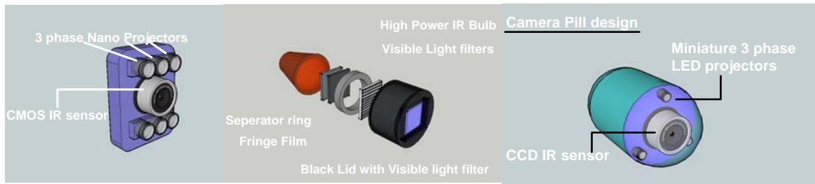
Fig 4.4 3D webcam design using 3 phase nano projector, car sensor for obstacle detection and camera pill design
