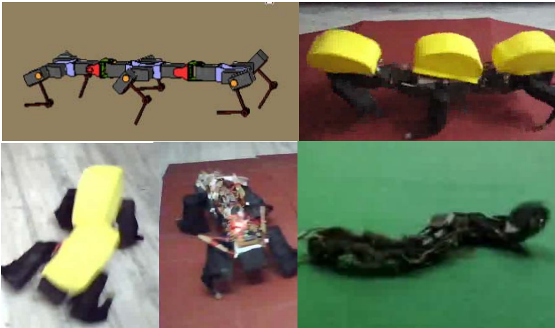
Fig 5.8 Modular legged design showing 4 legged robotic dog, a hexapod and a snake robot
