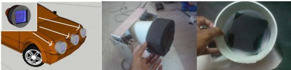
Fig 4.3 Outdoor version of the sensor using an IR medical bulb
