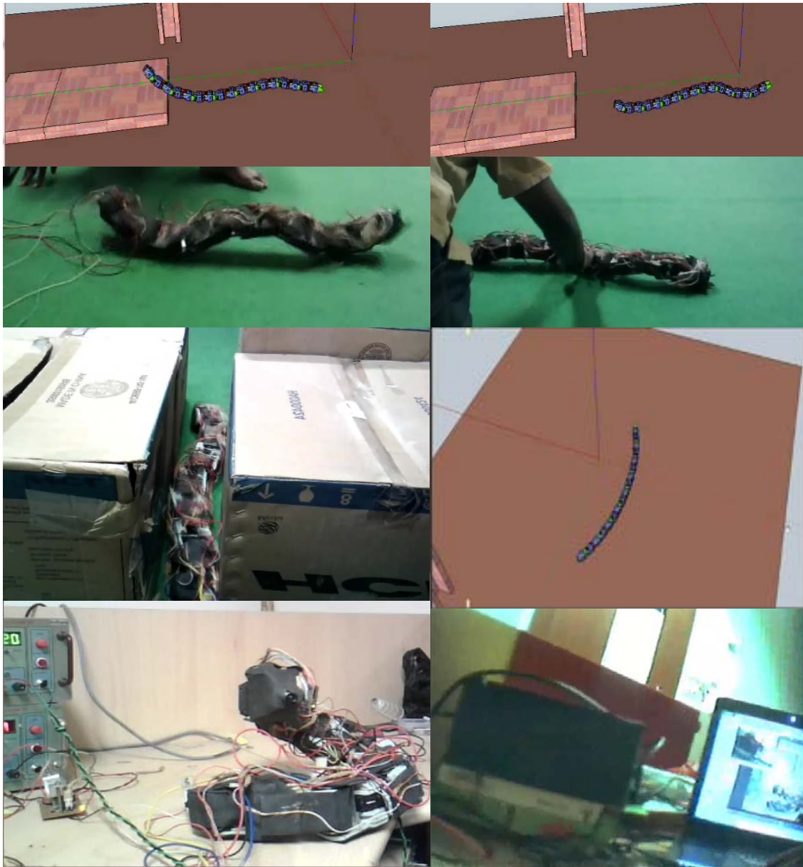
Fig 5.5 Snake P2 gait simulations, crawling through a passage and camera snooping
