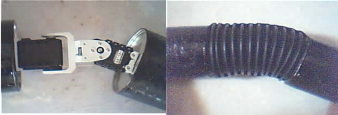
Fig 5.2 2 d.o.f orthogonal modular unit usgin Bioid AX-12 servos and bellow design
