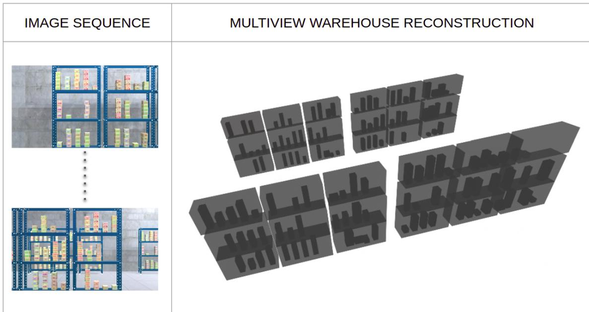
Figure 3.9: **Multi View Reconstruction** of the entire warehouse using four sequences covering 280 frames (70 frames each), using the layouts predicted by *MVRackLay-Disc-4*.
