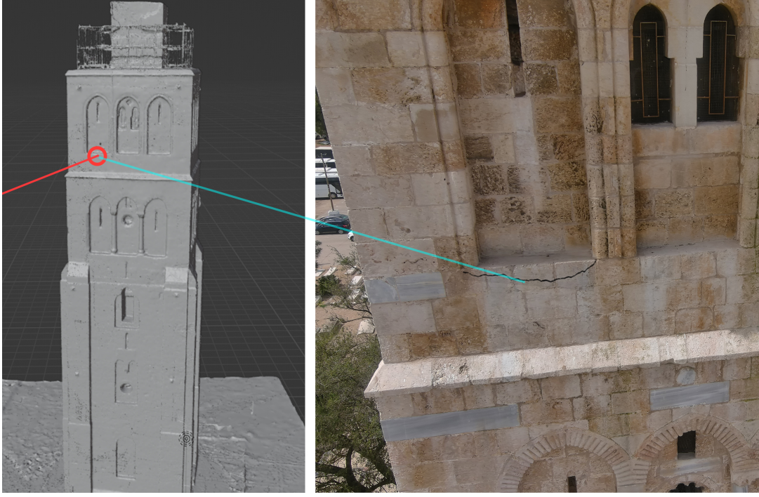
Figure 3.4 3D mesh model of the building (left) using 2D to 3D mapping shown using the red ray and red ring; Captured image of the building (right) using UAV showing 2D image of it. Correspondences of all the three images are shown using blue lines.
