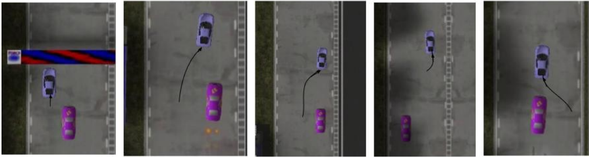
Figure 4.1: Results of blocking behavior, in first three images, the purple car moves towards right to overtake our(blue) agent, our agent also moves towards the right to prevent the overtaking. In last two frames, the purple car is translating towards left and back to center and our car, also translates in center to block it from overtaking.
