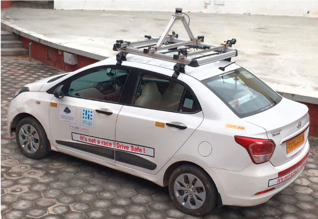
**Figure 2.1** The vehicle with all available sensors mounted. The LiDAR is mounted at the top of the car, and the 6 cameras are arranged in the configuration as front, front-left, front-right, back, back-left, and back-right. The GPS sensor is mounted towards the rear screen. All sensors are connected to a USB3 hub inside the car which is then connected to the on-board computing machine and storage.
