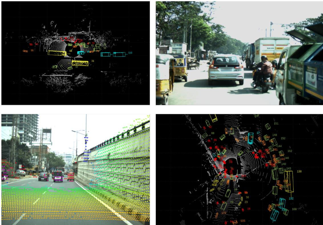
**Figure 3.1** Some examples from the dataset showing different traffic scenarios, LiDAR data with annotations, and a sample of LiDAR point clouds projected on camera data.
