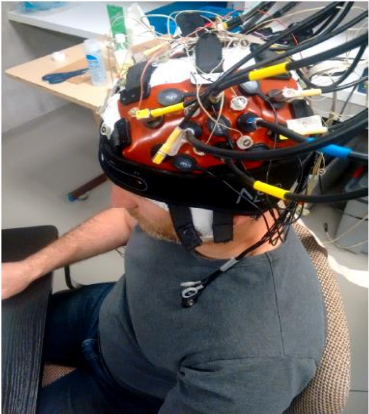
Fig 5.2 Illustrative example of the fNIRS-EEG/HD-tDCS set-up (red ellipse) overlying the left primary sensorimotor cortex (SMC).
