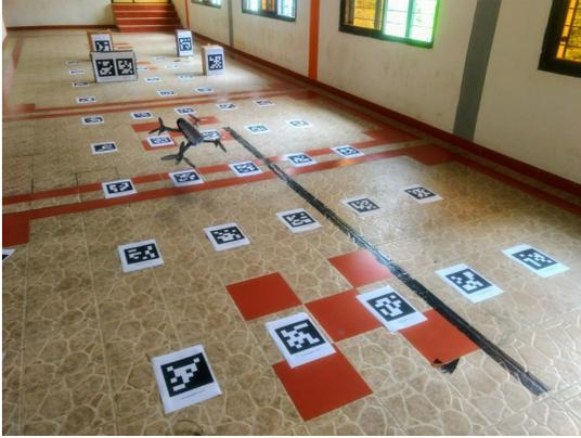
(a) Experimental setup with Apriltags arranged as a grid for ground truth.
