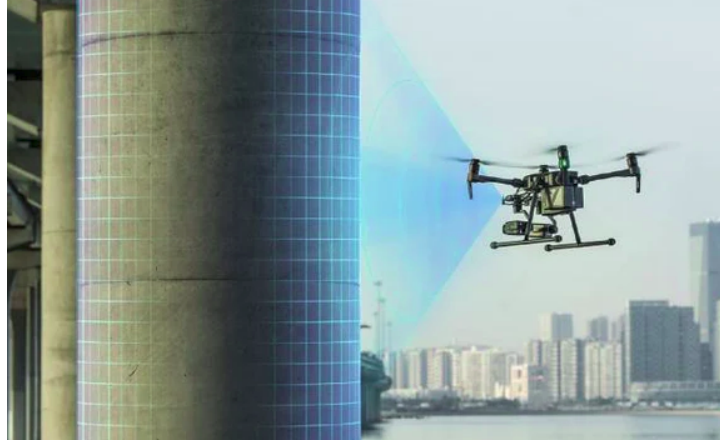
Figure 1.2: Shows current use of UAVs for inspection tasks near bridges. Source: https://candrone.com/pages/inspection
