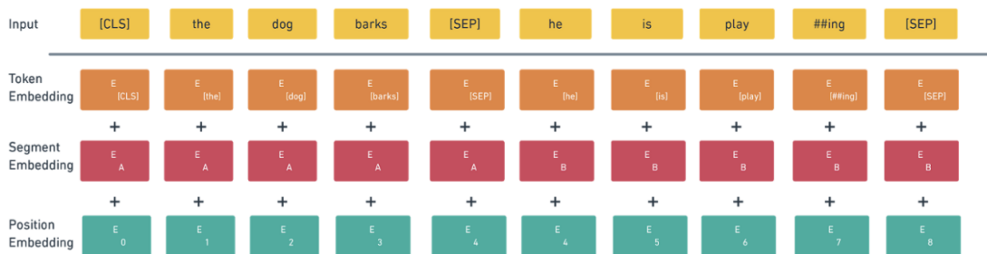
Figure 2.1 The input embeddings in BERT are made up of three separate embeddings
