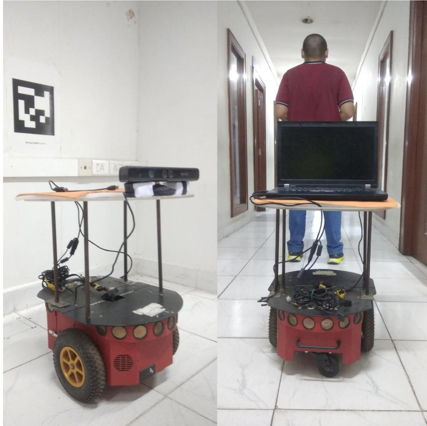
Figure 1.2: PFR- A Real-World Simple Prototype. Left: P3DX front-view with mounted RGBD Microsoft Kinect. Right: P3DX rear-view with control computer with a target person in view.
