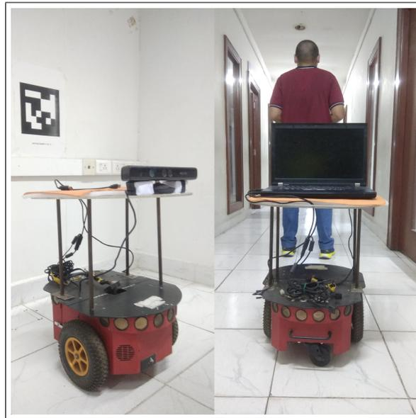
Figure 5.9: Our Configuration of P3DX 2-Wheeled Drive with Mounts
