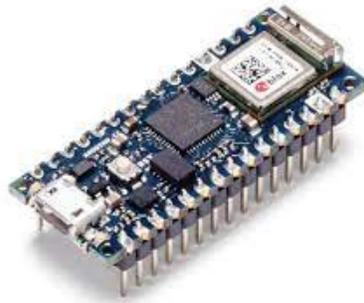
Figure 2.3: Arduino Nano 33 IoT used in our final version
