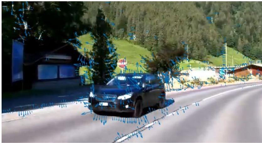
Figure 2.5: Optical flow vectors from Lucas Kanade Algorithm
