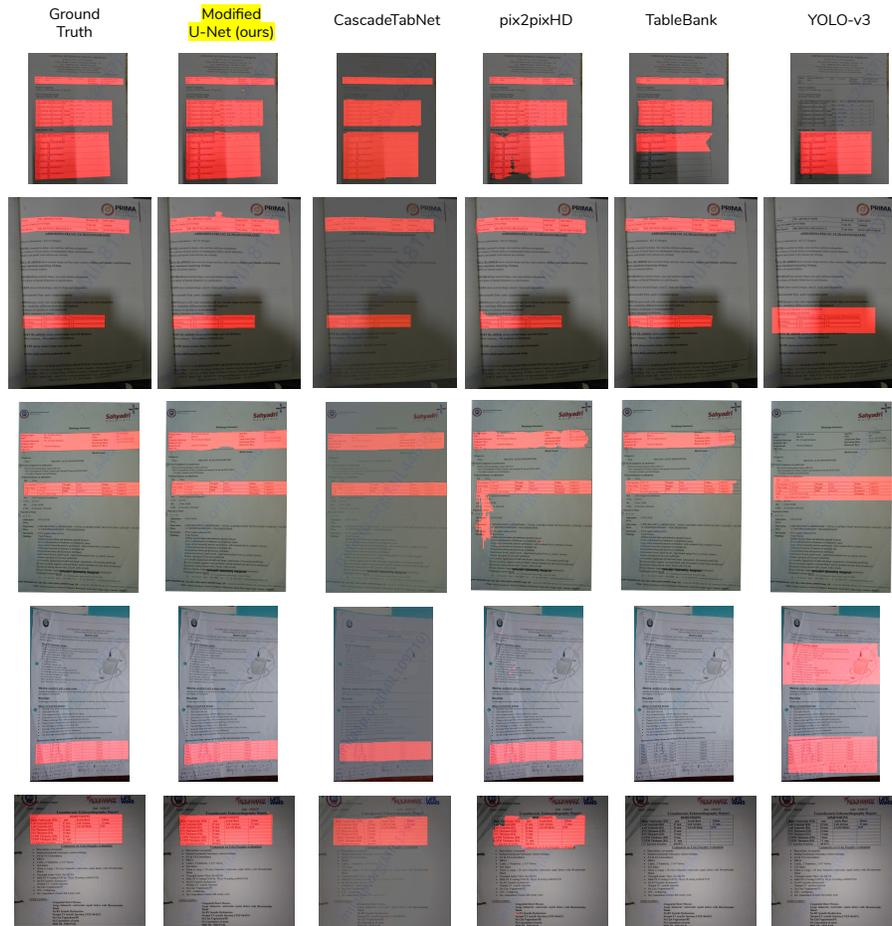
Fig. 3: Table localization results for various models for images with highest IoU score using our model’s predictions.
