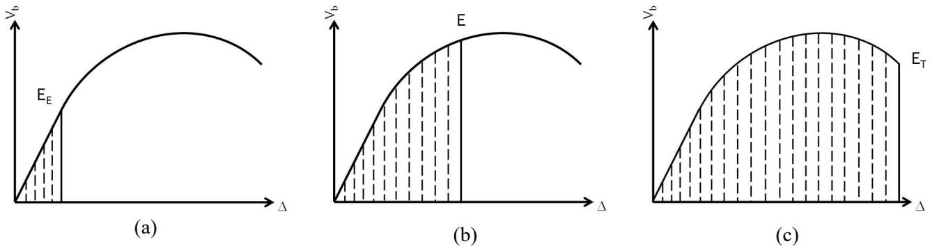
Fig. 5 – Estimation of energy-based damage from capacity curve [16]
