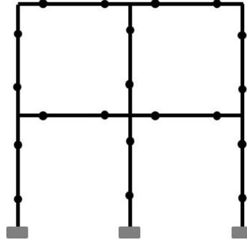
Fig. 4 – Assigned hinge locations for beams and columns
