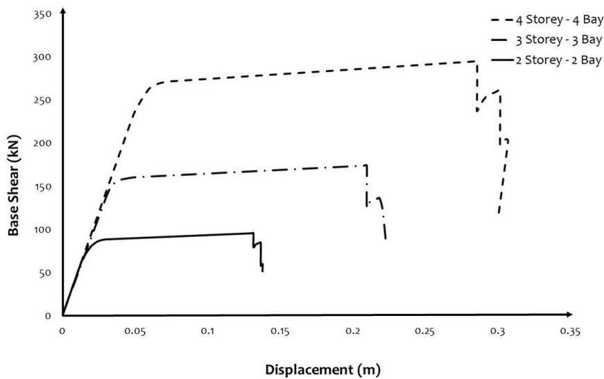
Fig. 6 – Capacity curves of Ideal Frames
