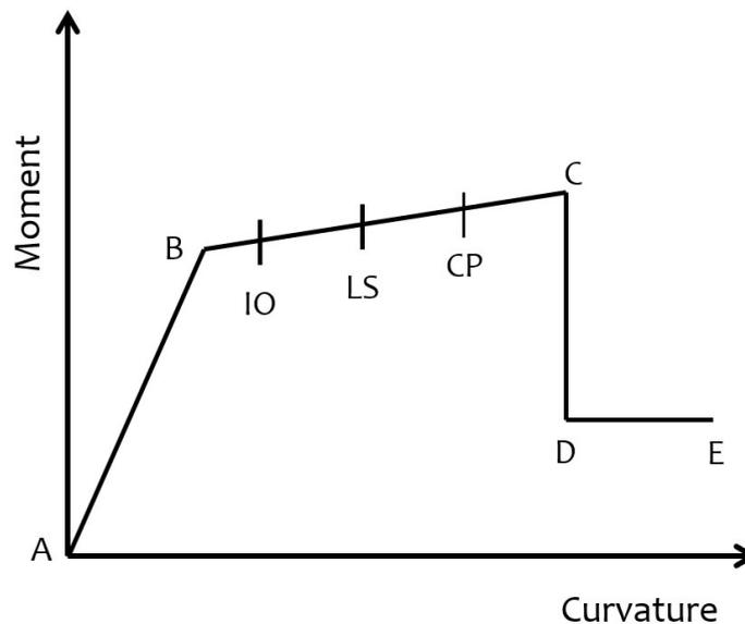
Fig. 2(a) – Typical moment curvature relationship of a hinge
