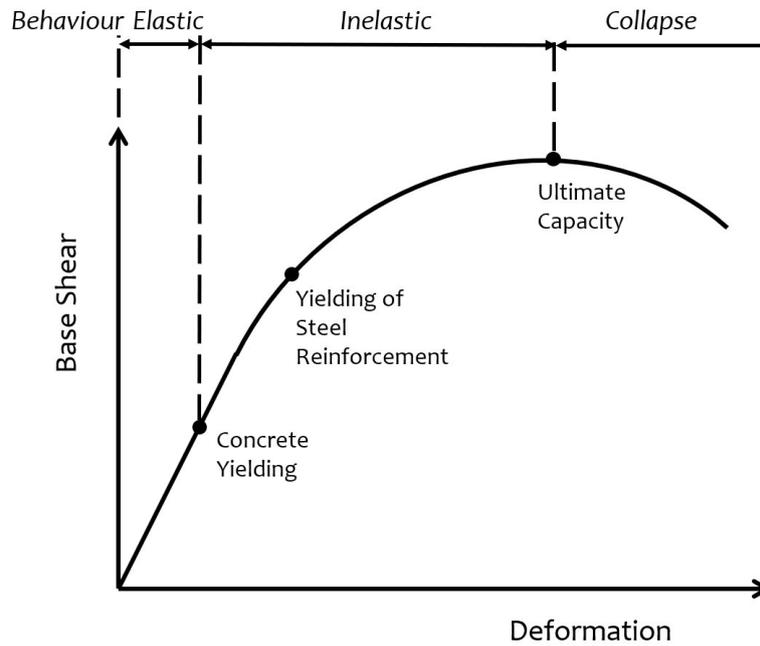
Fig 1 – Typical structural performance and associated damage state
