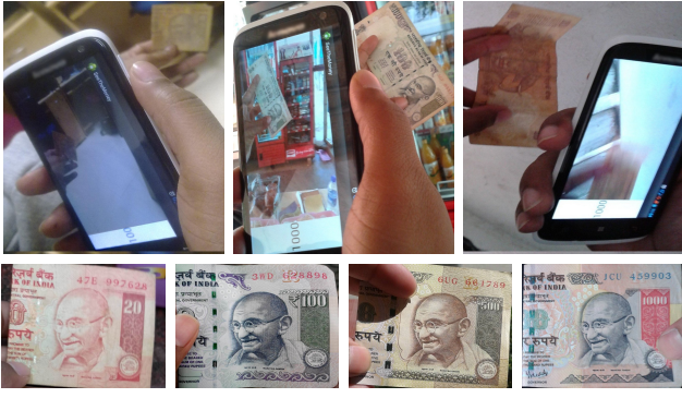
Fig. 9: First row: Failure cases. On the left and middle, the bill occupies less than 40% of the image, leading to a segmentation failure and incorrect response. On the right, the image captured is highly blurred. Second row: The obverse (front) side of bill showing the portrait of Mahatma Gandhi which is common in every denomination. There are very few distinguishing features on this side.
