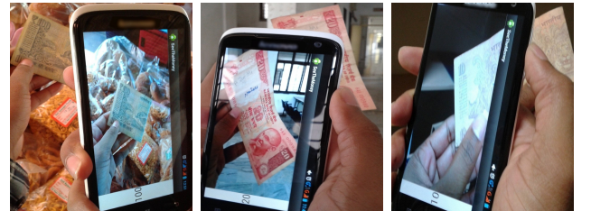
Fig. 8: Currency recognition application at work in various configurations and environments. The application gives a correct result for all the cases.
