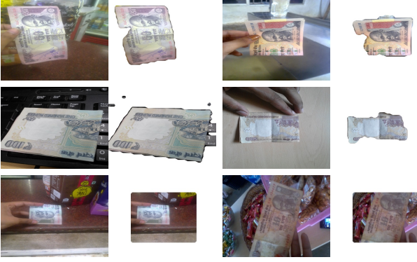
Fig. 3: Segmentation on a currency bill. The first and second rows show successful segmentation results while the last row shows segmentation failure where center region is marked as foreground.
