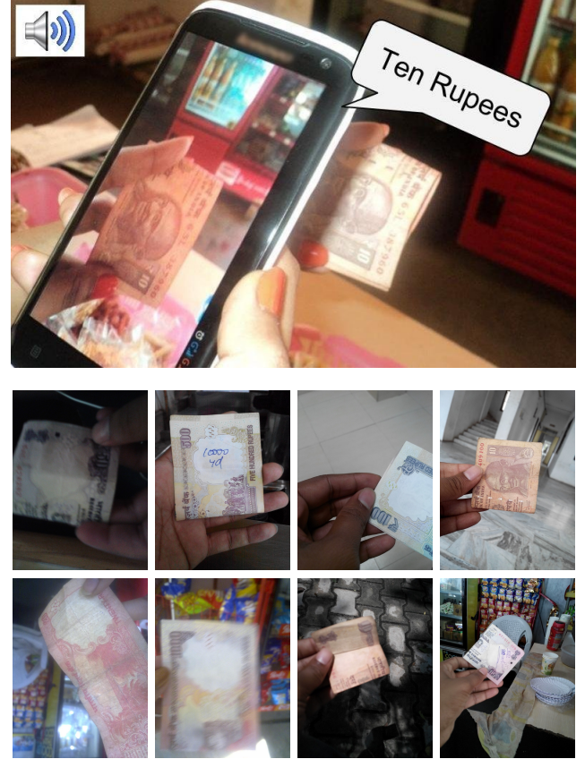
Fig. 1: The top row shows a typical use case of our currency recognition app. Our application recognizes a bill from an image with many distracting objects and speaks it out. The last two rows show images from the dataset for Indian National Rupee (₹), with bills in varying illumination and background.
