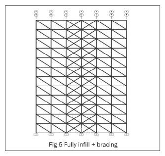
This frame consists of fully infill frame retrofitted with bracing. This frame is only considered to study the effect of addition of bracing to the frame.
