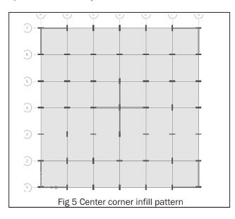
In this type of building infill are provided in center and corner part of the building as shown above.
