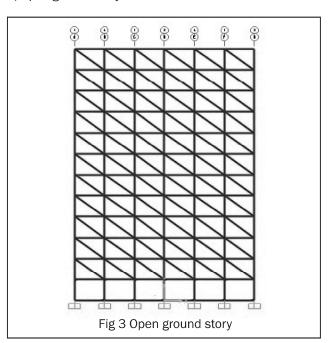
This building consists of infill wall on all floors except for ground floor. The paper mainly studies the impact of removal of infill from ground floor. This is a practical case made to study impact of removal of infill from the ground story of the building.
