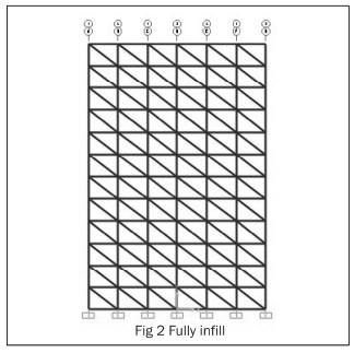
In this frame the building is modeled with infill throughout the building this case is considered for analytical study of difference between bare and building with open ground story. This frame consists of infill masonry wall throughout the frame in order to study the impact of it on the capacity of the building.
