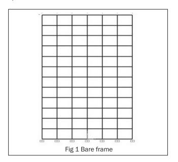
This frame consists of column beams and slabs. Wall loads are considered over beams. No additional modeling for wall is considered in this frame i.e. no additional stiffness of wall is considered in entire frame.
