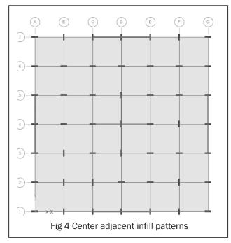
In this type of building infill are provided in center and middle part of the outer building as shown above, this type of pattern is taken into consideration as few buildings are constructed with partial infill walls on the ground floor. This pattern mainly considers infill in particular location to study the impact of infill on the open ground story.
