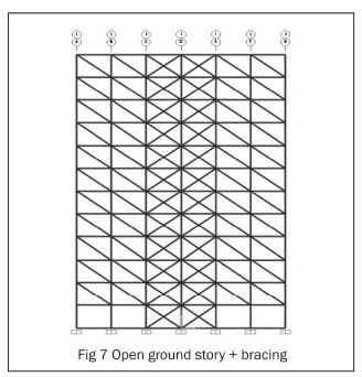
This frame is actual case which studies the effect of retrofitting open ground frame with bracing system. The bracing systems are provided over middle part of outer frame.
