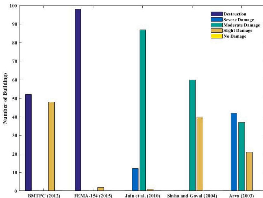
Fig. 6. Comparison of RVS results for sample 100 surveyed RC buildings in Pithoragarh city.
