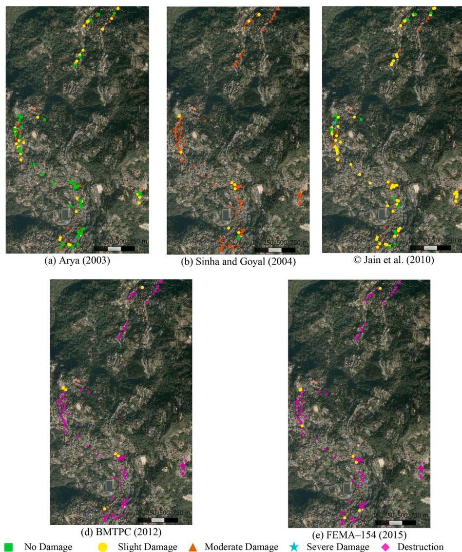
Fig. 8. Damage scale distribution of surveyed buildings with different RVS methods in Gangtok city.
