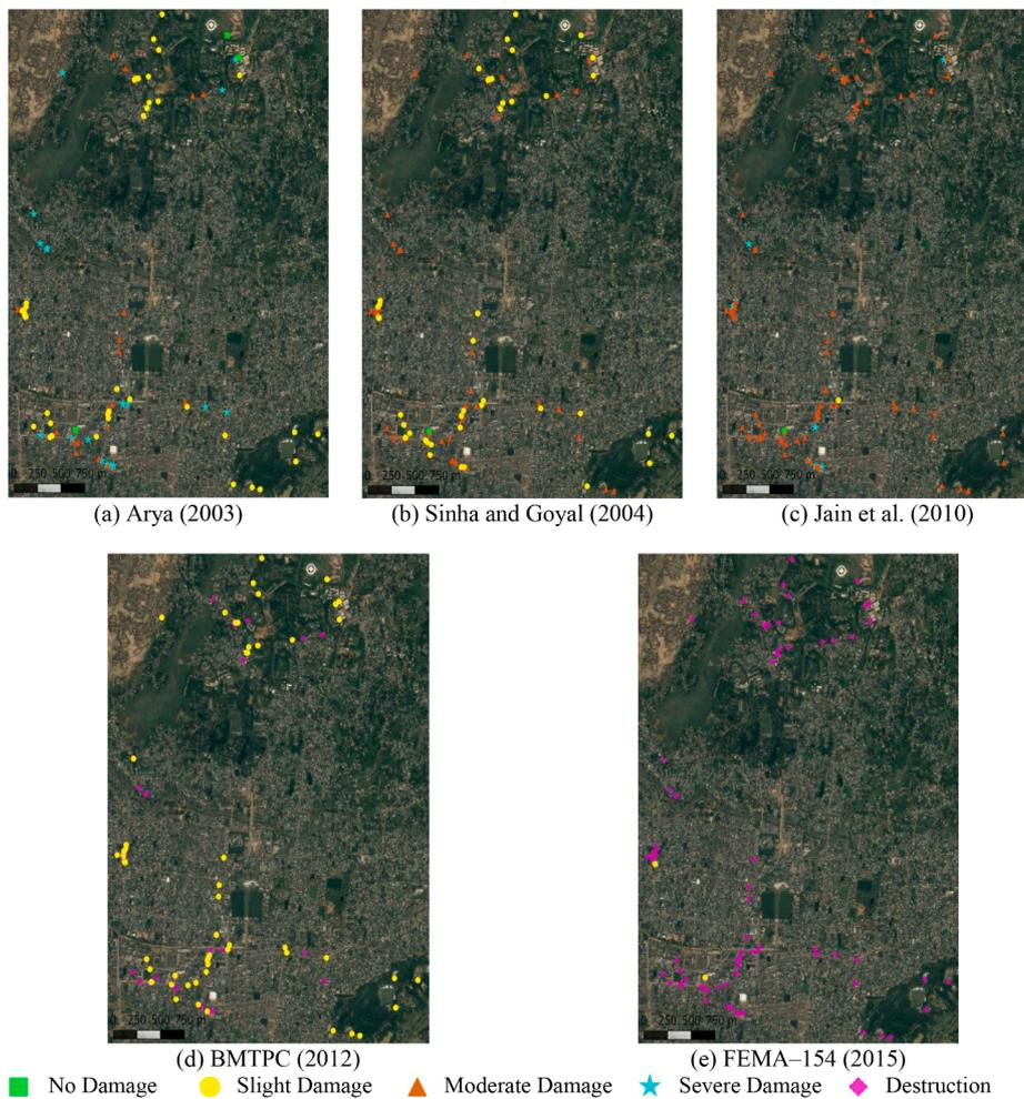
Fig. 10. Damage scale distribution of surveyed buildings with different RVS methods in Agartala city.
