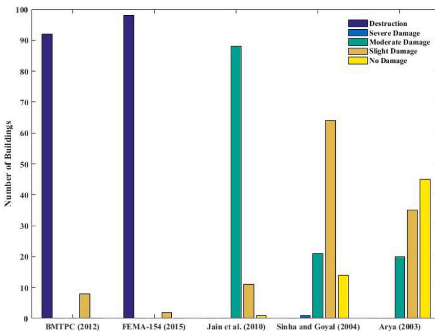
Fig. 7. Comparison of RVS results for sample 100 surveyed RC buildings in Gangtok city.
