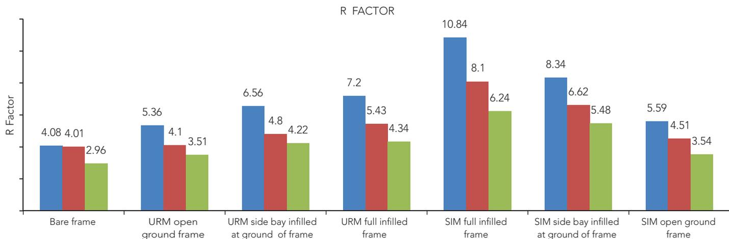
Figure 10: R-factor of different frames for different aspect ratio
