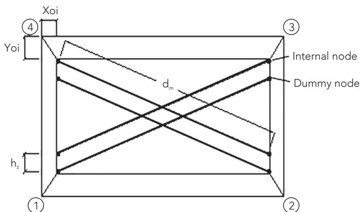
Figure 5: Inelastic infill panel element
