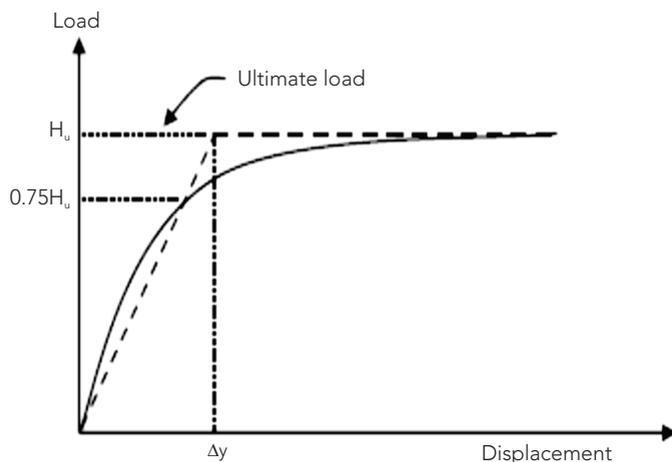
Figure 3: Reduced stiffness method
