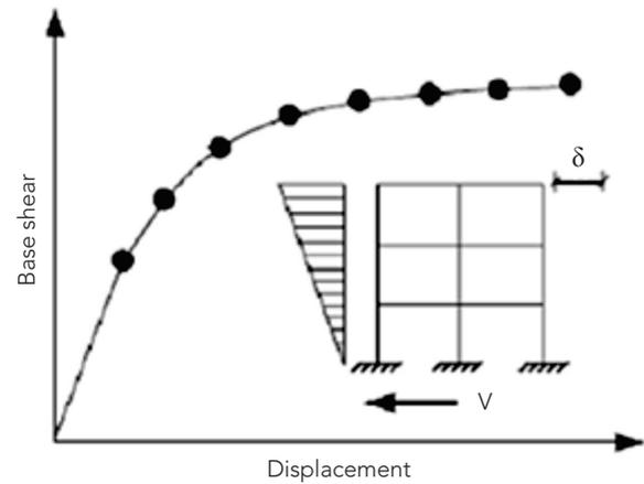
Figure 6: Capacity curve
