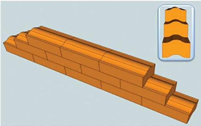
(a) Semi-interlocked masonry
