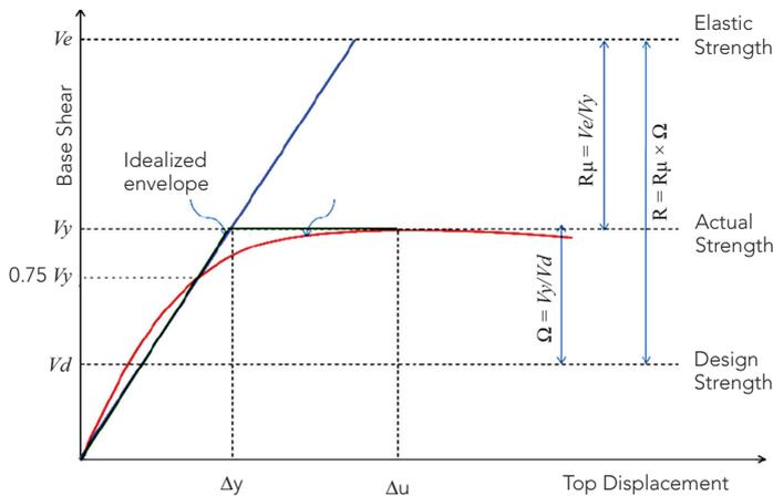
Figure 2: Relationship between response reduction factor, structural over-strength ( $\Omega$ ) and ductility reduction factor ( $R_\mu$ )<sup>[4]</sup>
