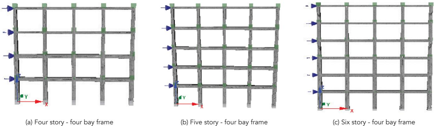
Figure 4: Different two dimensional frames
