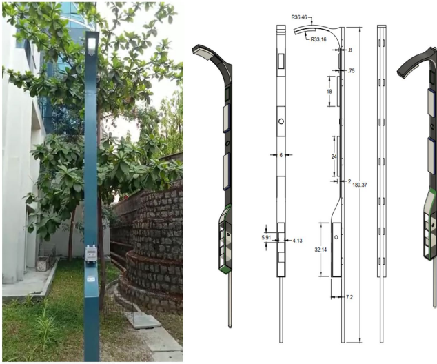
Fig. 4. a) One of the smart lamp posts deployed in the IIIT-H campus b) The design of the fabricated smart lamp post. Several compartments has been provided at the bottom and midway to house nodes with sensors. All measurements are in inches.
