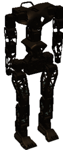
Figure 1 27 DoF humanoid robot with articulated torso.
