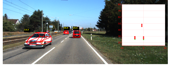
Fig. 1. Example output from the proposed monocular object localization system. The system is capable of estimating the shape and pose of dynamic objects in real time. The image shows the estimated shapes (wireframes) projected onto the image. Above each of the wireframes is a depth estimate to the object. The inset plot shows the top view of the localization output (red) overlaid on the ground truth (green). Even objects 50 meters are accurately localized.
