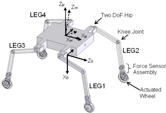
Fig. 1. Mechanical Structure of the HWLV
