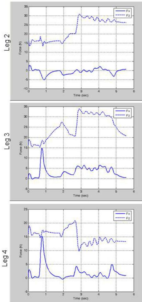
Fig. 11. Horizontal and vertical forces measured by force sensor on leg2, leg3 and leg4 during step climbing by leg1
