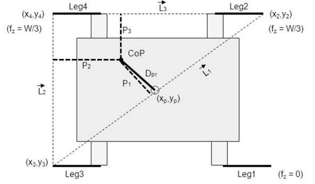
Fig. 6. Center of Pressure (CoP) with leg2, leg3 and leg4 in contact and in nominal position
