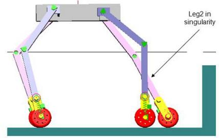
Fig. 7. Leg2 reaching workspace singularity before chassis reaches the desired position
