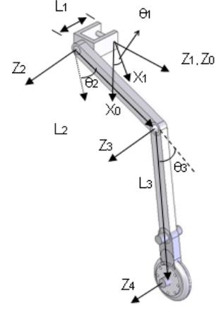
Fig. 2. Kinematics of the single leg chain
