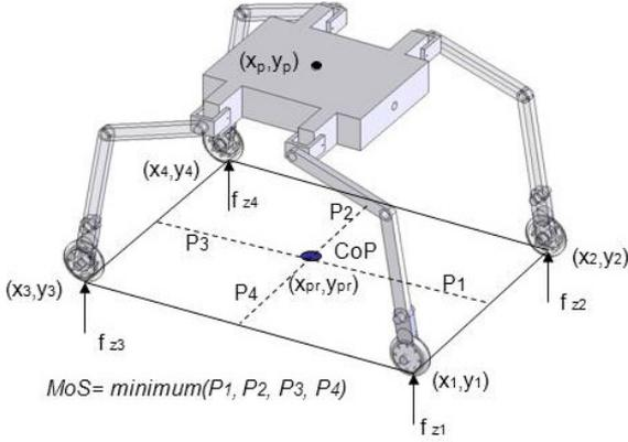
Fig. 5. Centre of Pressure (CoP) and Margin of Stability (MoS) with all legs in contact
