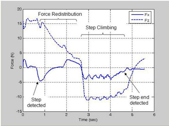
Fig. 10. Horizontal and vertical forces measured by force sensor on leg1 during step climbing sequence
