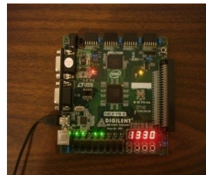
Figure 7: Xilinx Nexys 2 Development Board with Spartan 3E FPGA
