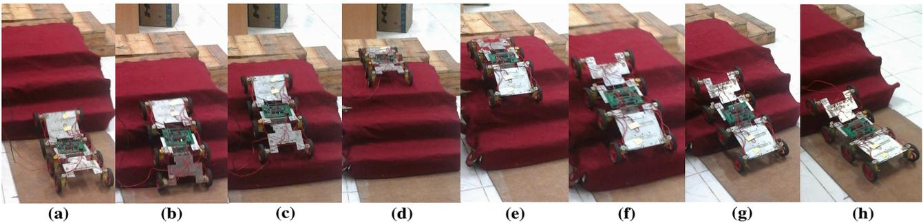
Fig. 18: Stages (a)-(d)The robot is ascending and in (e)-(h) descending on carpet stairs with dimensions as 12cm riser height and 18cm tread width
