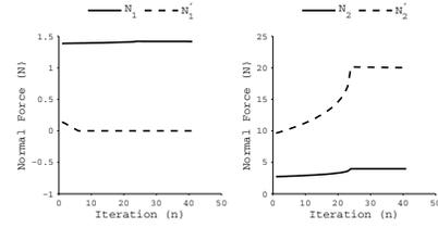
Fig. 4: Normal Force for (a) Wheel-1 and (b) Wheel-2 without (Block line) and with (Dashed line)  $k_1^-$  and  $k_2^+$
