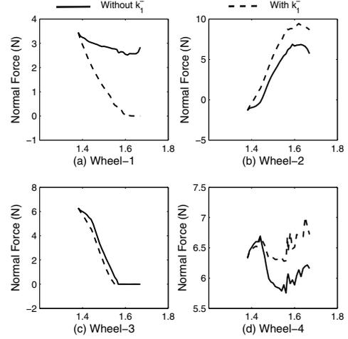
Fig. 10: Graphs depicting the Normal Forces at all the wheel-pairs for cases with spring of stiffness  $k_1^-$  (dashed) and without it (solid)
