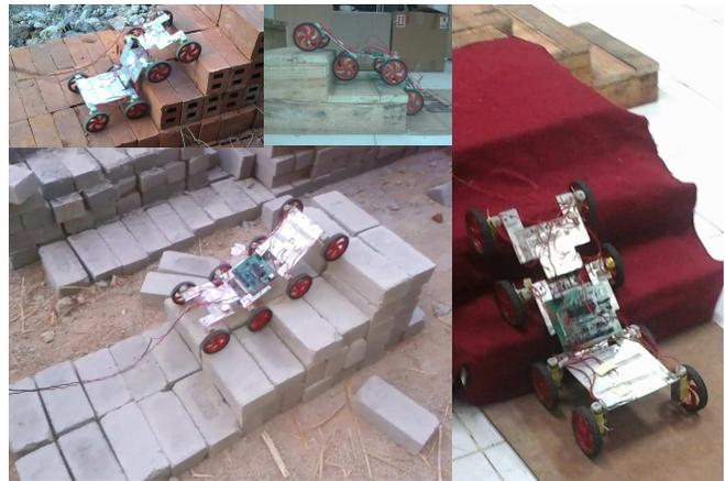
Fig. 1: Compliant modular robot prototype
