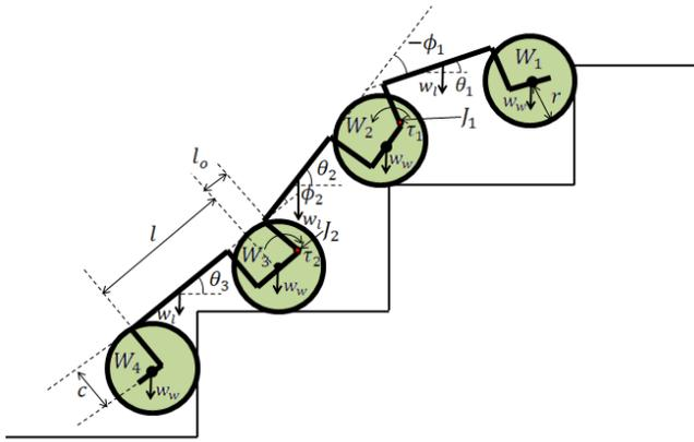
Fig. 2: Schematic of the 3-module robot
