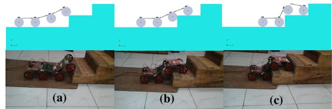
Fig. 14: Numerical Simulation and Experimentation on robot with only one spring( $k_1^+$ ) at Joint  $J_1$
