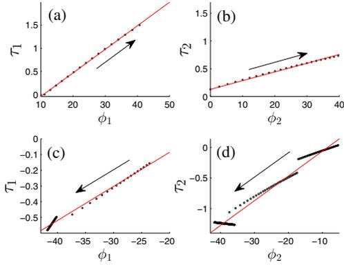
Fig. 9: Moment Profile ( $\tau_i$ ) obtained at : (a)  $J_{i=1}$  for increasing profile of Joint angle  $\phi_1$  for  $k_1^+$  (from Phase-1) (b)  $J_{i=2}$  for increasing profile of Joint angle  $\phi_2$  for  $k_2^+$  (from Phase-3) (c)  $J_{i=1}$  for decreasing profile of Joint angle  $\phi_1$  for  $k_1^-$  (from Phase-2) (d)  $J_{i=2}$  for decreasing profile of Joint angle  $\phi_2$  for  $k_2^-$  (from Phase-3)
