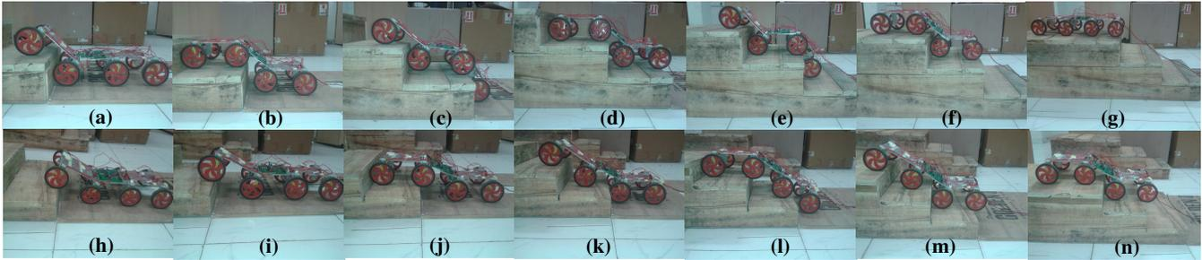
Fig. 15: Stages (a)-(g)The robot is ascending on stairs with dimensions as 11cm riser height and 22cm tread width and Stages(h)-(n) as 8cm riser height and 18cm tread width
