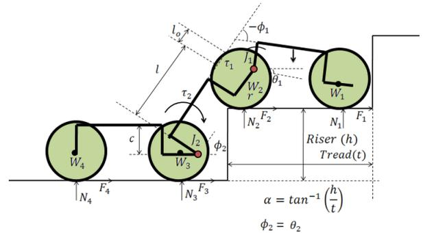
Fig. 3: The robot getting stuck while ascending stairs with only one spring at  $J_1$
