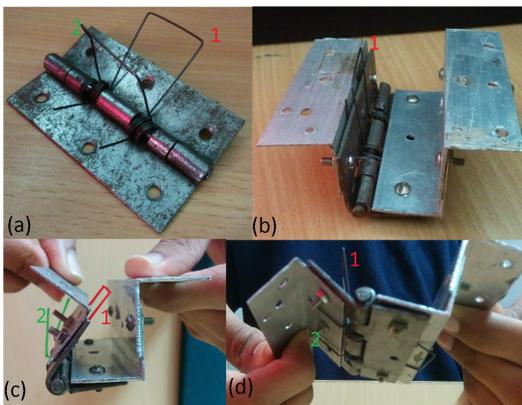
Fig. 13: The Spring Assembly -  $k^+$  is labeled as (1) and  $k^-$  is labeled as (2) : (a) Spring loaded hinge, (b) Joint with mounts for the robot, (c)  $k^+$  in action and (d)  $k^-$  in action
