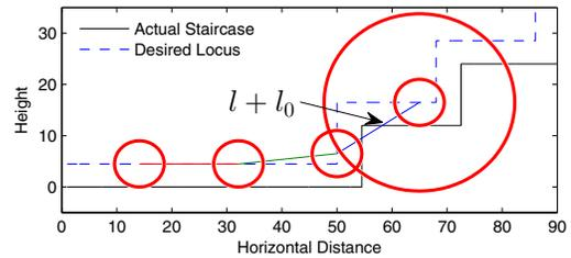
Fig. 5: Demonstration of finding Wheel center of Wheel-2 when given the wheel center of Wheel-1.
