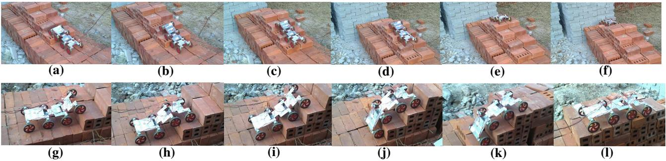
Fig. 17: Stages (a)-(f)The robot is ascending and descending on redbrick stairs with dimensions as 8cm riser height and 22cm tread width and Stages (g)-(l) with dimensions as 11cm riser height and 16cm tread width
