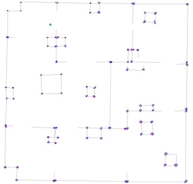
Fig. 8. EKF-SLAM results with Data association using MECPs, the lines in grey are drawn to correlate the SLAM results with the environment, the red plus symbols represent the mean of each feature and the blue ellipses around them represent their variance
