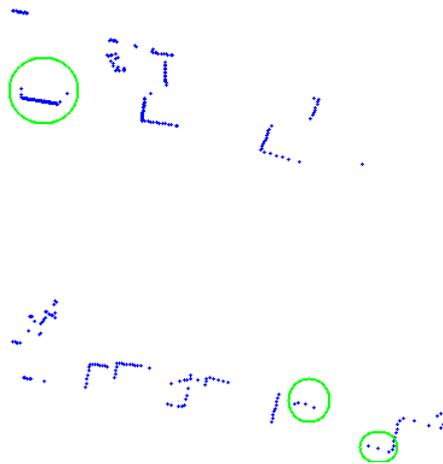
Fig. 2. Raw scan data, the laser points inside the green ellipses are sparse
