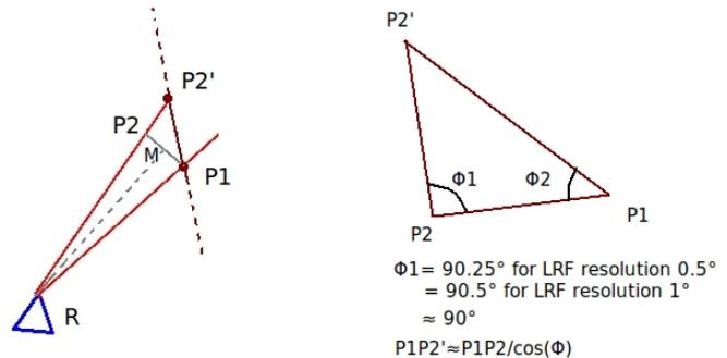
Fig. 1. Adaptive Clustering Threshold
