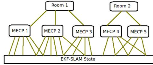
Fig. 6. The Hierarchy of data association, Data within a room can only be associated with other data from the room. Convex polygons from the same room can share vertices and edges, but Convex polygons from different rooms do not have any common vertices
