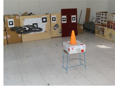
Fig. 3: Ardrone [3] performing 3D collision avoidance with obstacle (orange cone) by generating trajectories on-line through a sequence of collision free way-points. ArTags [18] were placed at strategic(predefined) location in flying area of the lab.
