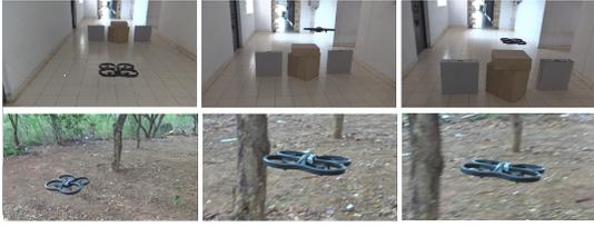
Fig. 9: Quadcopter avoiding obstacles based on obstacle detection using depth map
