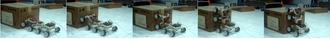
Figure 12: Snapshots of the robot climbing, a 30 cm high step
