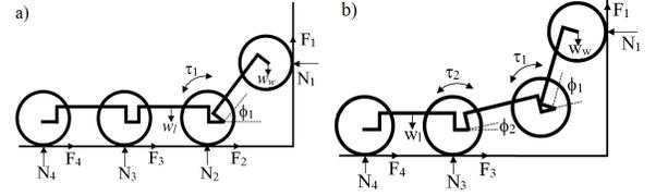
Fig. 4. Depiction of static forces and moments acting on the robot: The forces and moments are shown for the two possible climbing configurations i.e., a) Phase-1: when only one module is climbing and b)Phase-2: when two modules are climbing
