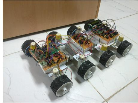
Fig. 1. A snapshot of the 3-module compliant robot prototype.
