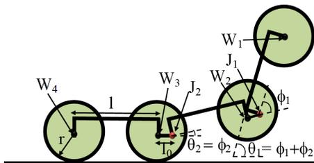
Fig. 2. The front view of the robot showing the trunk and wheel joints. The relative angles ( $\phi$ 's) and absolute angles ( $\theta$ 's) are also depicted.
