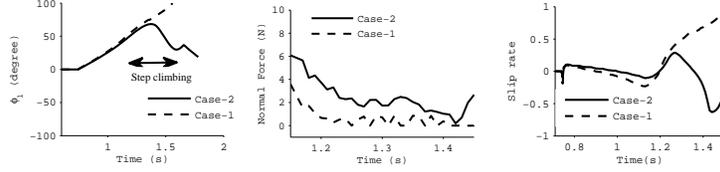
Fig. 7. Plots to analyze robot's climbing behavior while climbing a 14cm step: a)-c) The comparison of the joint angle ( $\phi_1$ ), normal force( $N_1$ ) and slip rate (at Wheel 1) between cases with spring (Case-2) and without spring (Case-1) at  $J_1$
