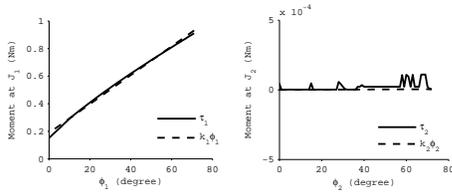
Fig. 5. Moment plots for joints  $J_1$  and  $J_2$ : The plot shows the desired moments obtained from the optimization procedure (solid line) and the moments generated by the optimal spring (dotted line). The slope of the dotted line yields the spring stiffness value
