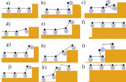
Fig. 6. Step climbing ability of the 3-module robot: a)-c) Case-1: the passive robot tips over while climbing a height of 14 cm; d)-f) Case-2: it successfully climbs the step of 14 cm using a compliant joint at  $J_1$ ; Case-3: g)-i) the robot with a compliant joint at  $J_1$  manages to climb a height of 16 cm but is unable to pull the remaining links; Case-4: j)-l) it is able to fully climb a height of 16 cm using compliant joints at  $J_1$  and  $J_2$
