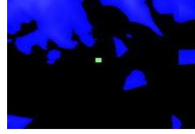
Fig.2 : Partitions in the exposure surface. Due to the presence of the outposts, the exposure surface need not always be contiguous. The green square indicates the outpost. The blue regions are the areas not visible to the outpost. UAV from one blue region cannot move into another blue region without becoming visible to the outpost
