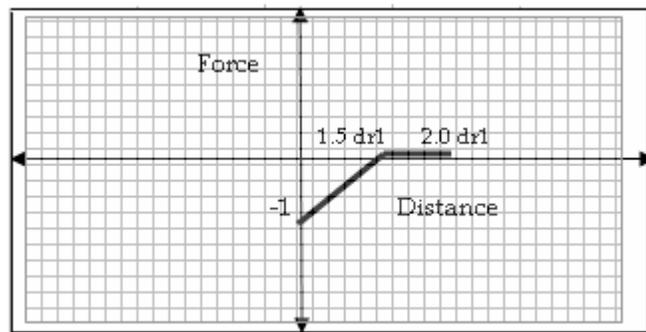
**Fig.2** Sensor-Obstacle force for Parker's algorithm.  $dr_1$  is the cutoff point for the sensor-sensor force in [12].
