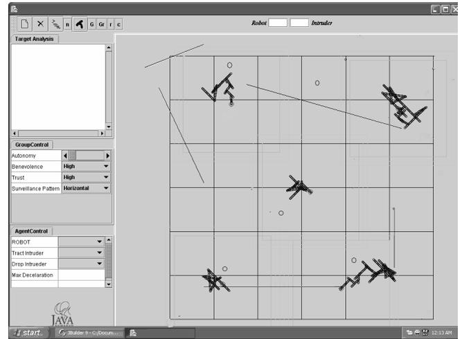
**Fig.2a** Snapshot of Krishna's algorithm in the known case. The sensor trails are the polygonal lines, and the black circles are targets.
