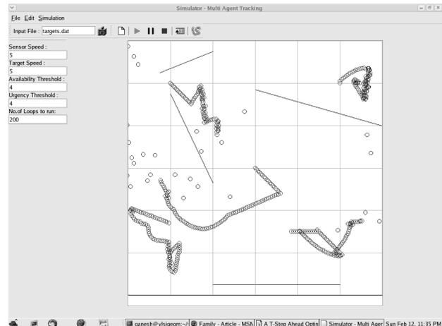
**Fig.2c** Sukhatme-Jung algorithm in the known case, the curved lines indicating the sensor trails, and the small black circles indicating the targets.
