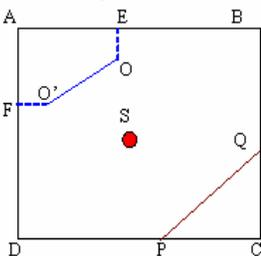
**Fig.1** Estimating the transit time for a polygonal cell.  $S$  is the sensor,  $OO'$  the obstacle,  $E$  and  $F$  the feet of perpendiculars from  $O$  and  $O'$  to  $AB$  and  $AD$ .  $P$  and  $Q$  are sample points in the FOV  $EBCDFO'O$ .
