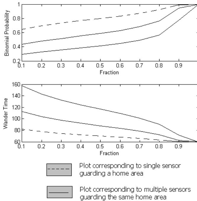
Fig. 7. Plots of individual probability and wander time against varying values of desired fraction  $f$ . Solid lines are plots corresponding to multiple sensors while dashed lines correspond to single sensor case. The lower and upper solid lines in the top graph and the upper and lower solid lines in the bottom graph correspond to scenarios where three and two sensors guard the same home area.
