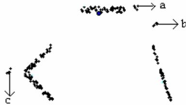
**Fig 5b:** Transient objects of figure 5a appear as outliers at 'a' and 'b'. Multiple reflections at corner 'c' of 5a appear as outliers at location 'c' in this figure
