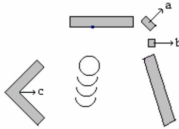
**Fig. 5a.** Simulation environment used for testing. Robot is shown in circles. 'a' and 'b' are transient objects that move away. 'c' is a corner where sensor errors are prone to occur
