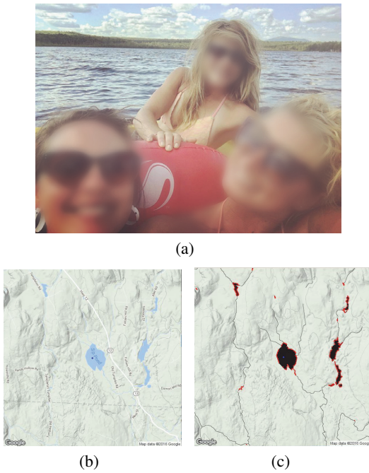
Figure 2: Segmentation Example: Different Stages of processing to get the final segmented image distinguishing between the water and land.
