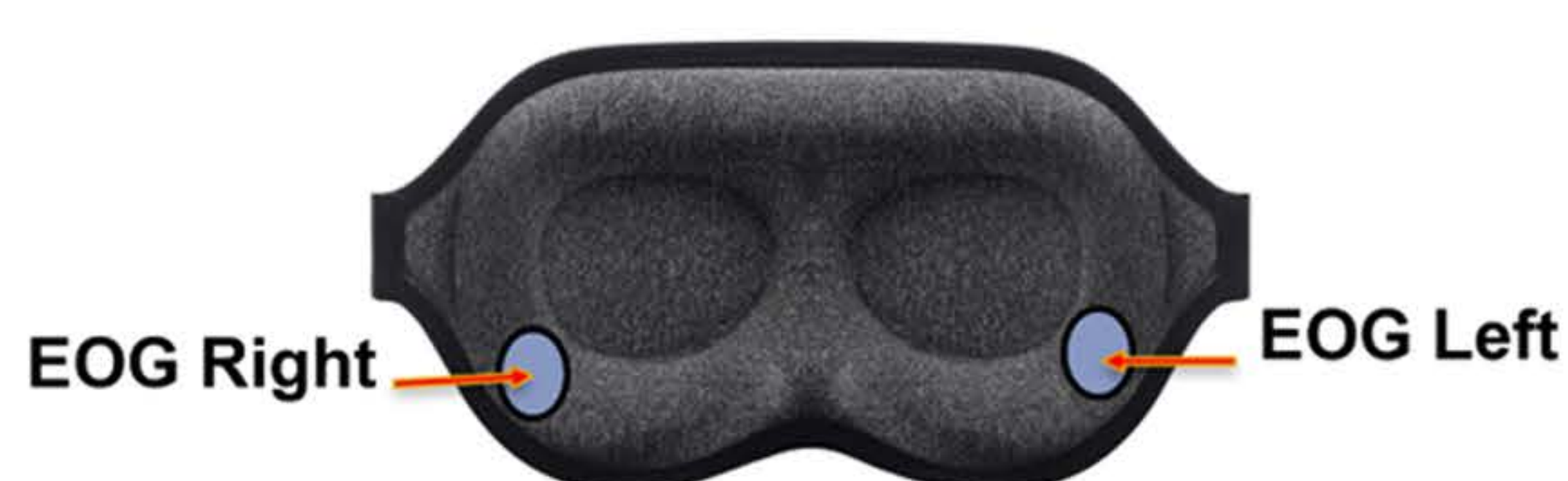
Figure 4: A sleep mask-based wearable device with one or two EOG electrodes (indicated by arrows) to capture eye movement data.
