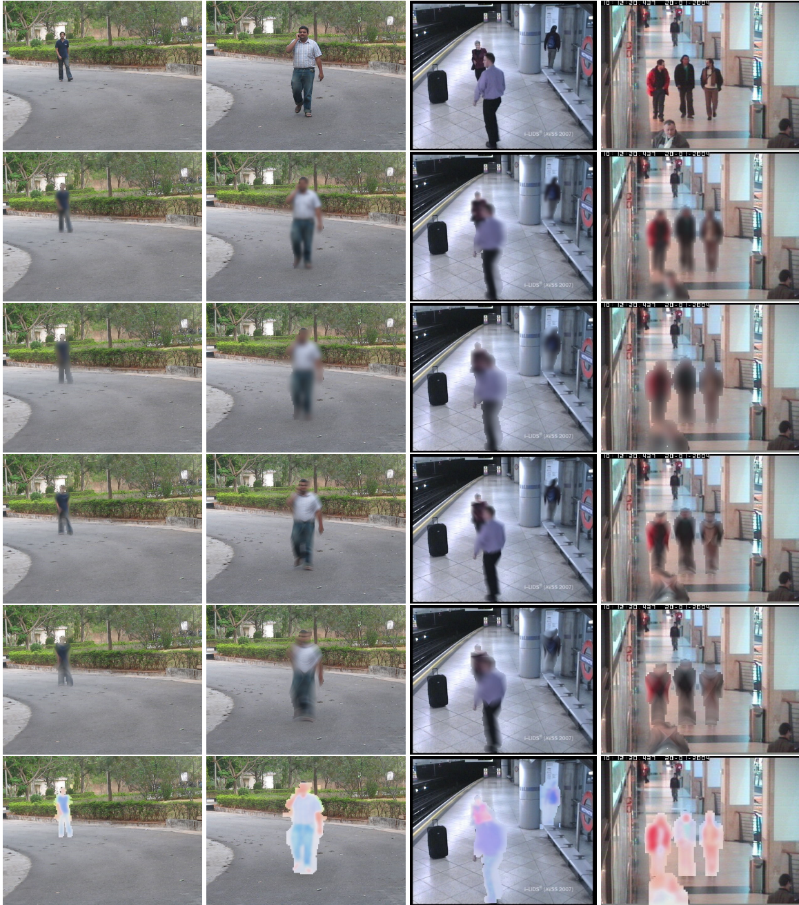
Figure 4.3 The first row shows the clear frames. The next five rows show the output of Blur-2, Blur-4, LIC-10, LIC-20, and Blur-2 followed by an intensity space compression, in that order.
