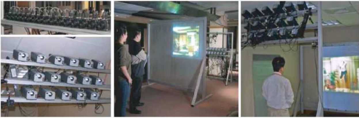
Figure 2.1: 3DTV :: Left: Array of 16 cameras and projectors. Middle: Rear-projection 3D display with double-lenticular screen. Right: Front-projection 3D display with single-lenticular screen.
