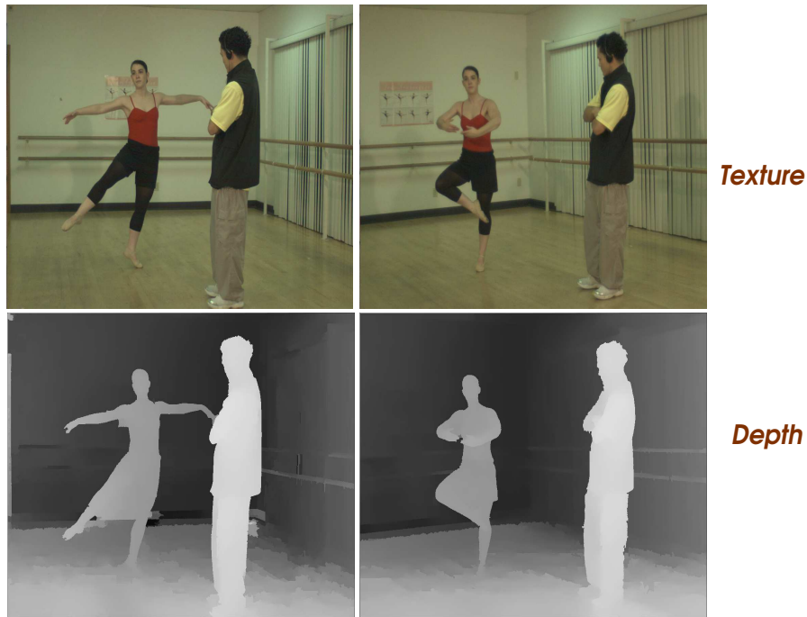
Figure 1.2: Texture (top) and depth map (bottom) of a scene at different time instant and from different viewpoint. [10]
