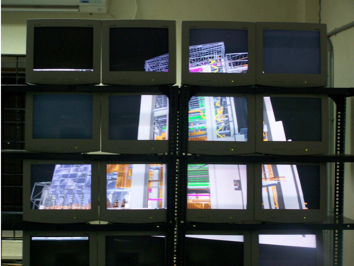
Figure 3.4 A 4 \times 4 display wall rendering of UNC's Powerplant. The combined resolution is 12 MPixels. Efficient rendering to a display wall requires fast visibility culling of the scene to all the frustums. Adaptive culling by merging of the object and frustum hierarchies makes this possible for even bigger tile configurations
