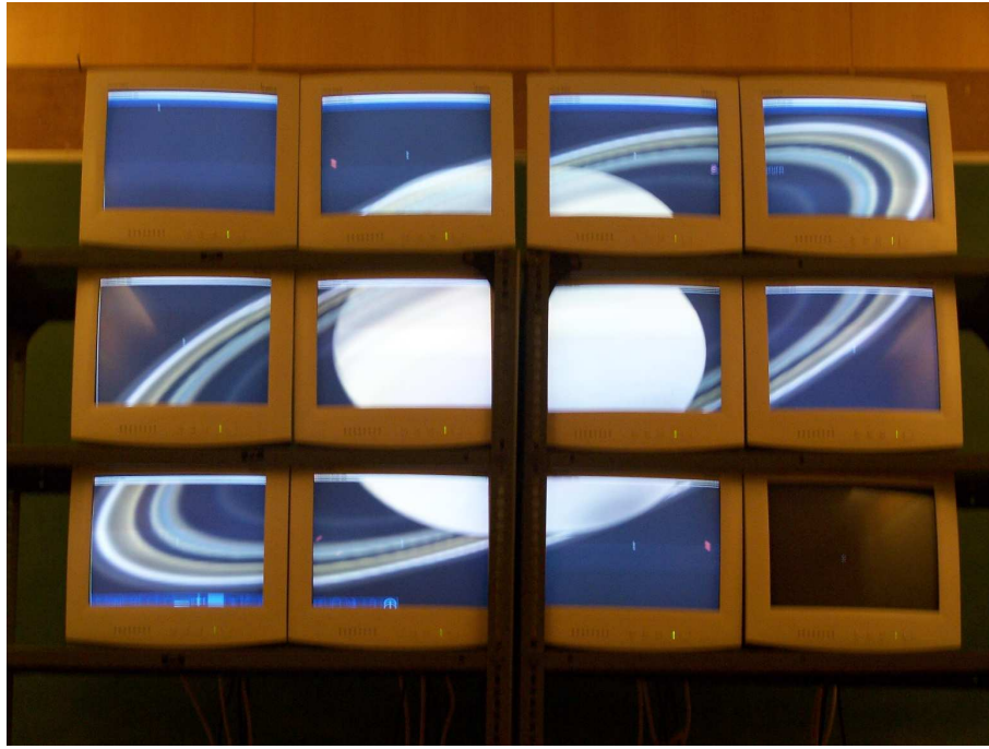
Figure 2.2 Chromium rendering a low-geometry model of Saturn over a 4 \times 4 tiled display wall.
