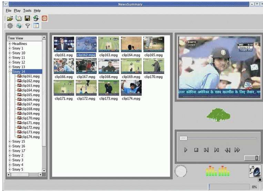
Figure 3.1 Detecting cuts in a broadcast news clip. A sports segment of the broadcast is illustrated here. The left panel shows a hierarchical structure of the video sequence. Key frames representing the shots in the video are shown in the middle panel, while the right panel shows a controller which plays the selected shot from the video.
