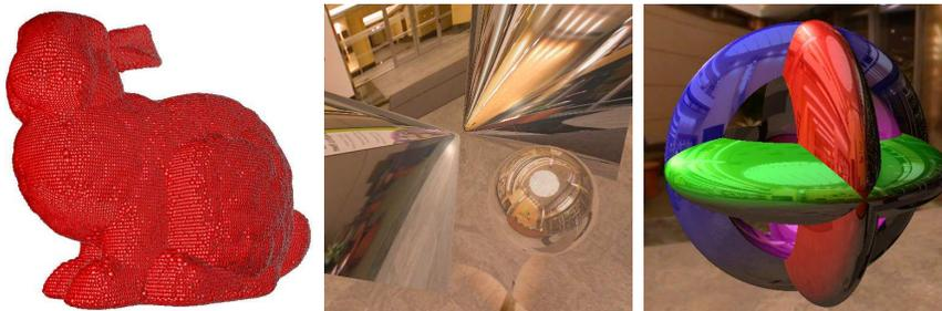
Figure 3.2: Left: Ray-traced Bunny model containing 36k spheres at 57 fps Middle: Hyperboloid ray traced with reflection and refraction at 300 fps Right: Four primitive CSG at 22 fps.
