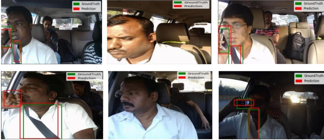
Figure 2.6: Phone Detection using YOLO model finetuned for the corresponding task. The green color box is for ground truth and red box is for prediction.
