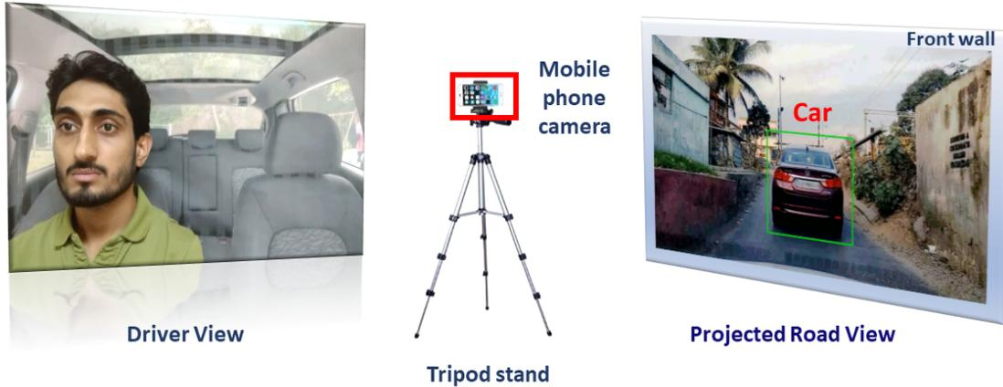
Figure 4.2: DGAZE Collection Setup: Dataset is collected in lab setting which has close proximity with actual driving setting. Mobile phone camera attached to tripod stand similar to mobile phone camera mounted on wind shield of the car collects both driver view and projected road view at same frame per seconds.
