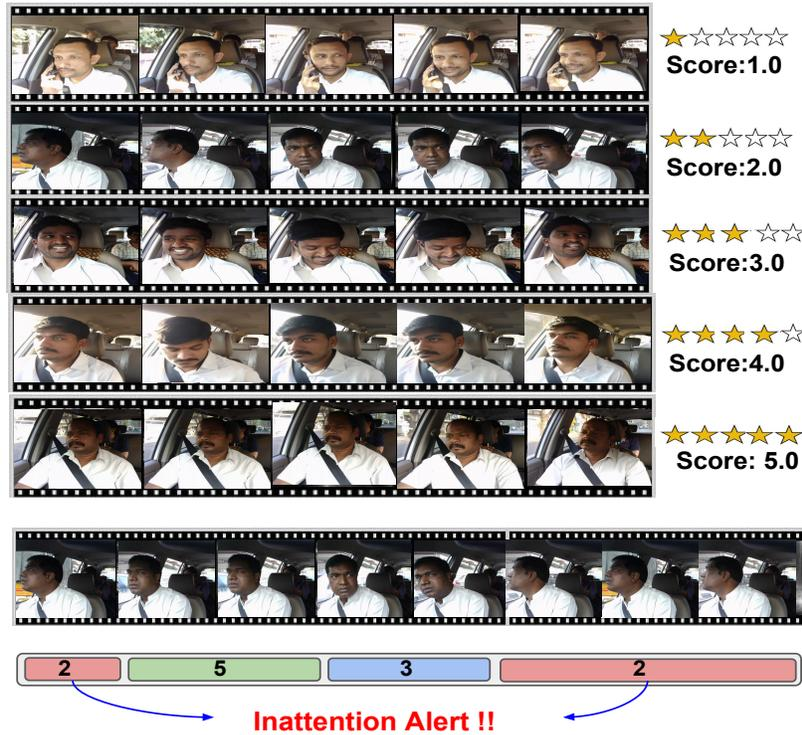
Figure 2.1: Rating system to predict driver attention based on specific and generic facial features. The figure on top shows the videos captured and annotated ratings. The figure at the bottom shows the use of AutoRate to predict driver inattention over a long video.
