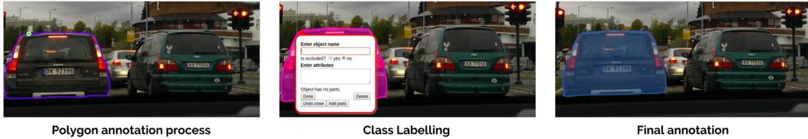
**Figure 2.4** A sample annotation for an image from Mapillary dataset on the web-based annotation tool, LabelMe. (left) is the annotation of an image in which an object is annotated with a polygon brush across its boundary; the circle in green is the control point to click when annotation for an object is completed. (middle) is the dialog box asking for the attributes of the annotated object along with its class label. (right) is the final segmentation mask of the object, car, in the image.
