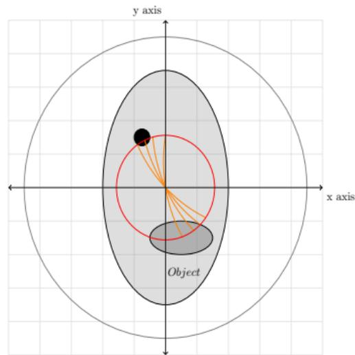
**Figure:** A sharp circular artifact is observed due to discontinuity in angular, as well as radial direction
