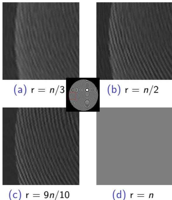
Based on our experiments, as a rule of thumb, dropping highest 10% of singular values gives a fairly stable reconstruction.
