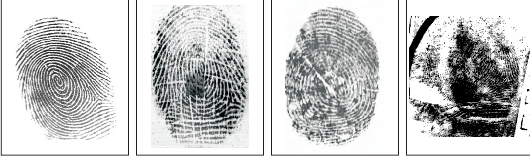
Figure 2.1 Fingerprint images of varying quality. From left: good quality; medium quality, distorted mostly by cuts; poor quality, varying moisture, cuts, and a lot of noise; latent fingerprint, taken from a crime scene, very little information.
