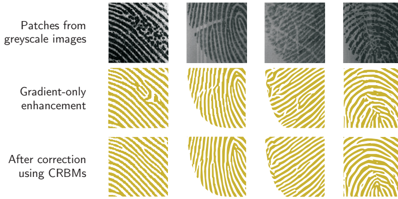
Figure 3.11 Examples of corrections in orientation fields and the resulting enhancements on noisy patches from some fingerprints. It can be seen that the corrections performed by the CRBMs remove local discontinuities in ridge structures. Further, they do not disrupt ridge structures that weren't noisy or distorted, thus indicating that the learning of local orientation fields was sound.
