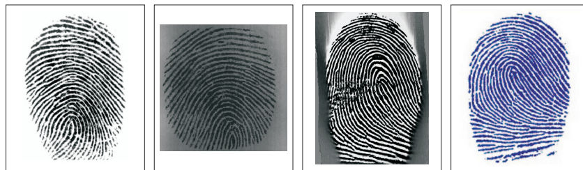
Figure 1.11 Fingerprints scanned using different types of scanners. From left to right: optical, capacitive, thermal and ultrasound. The thermal fingerprint was sensed using a sweep method, instead of a touch method. The sweep method requires the person to swipe his fingerprint over the scanner, instead of pressing down upon it. As a finger's surface reaches thermal equilibrium with the sensor surface very quickly, it is difficult to get a good print from the thermal scanner using the touch method.
