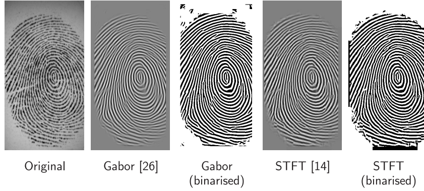
Figure 2.2 A fingerprint enhanced using Hong, Wang and Jain’s [26], and Chikkerur, Cartwright, and Govindaraju’s [14] algorithms. A binarisation is also performed on the enhanced image, by simply thresholding the enhanced image at its mean.
