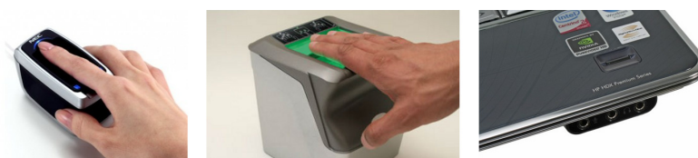
Figure 1.10 Some examples of fingerprint scanners. left : A single-finger scanner; centre : A multi-finger scanner; and right : A single-finger sweep scanner. Unlike the touch scanner, the sweep scanner asks the user to swipe his/her finger over it. This gives a sequence of overlapping slabs of the fingerprint image, which the scanner then stitches together.
