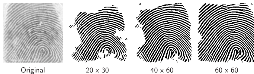
Figure 4.9 Reconstructions of the same fingerprint using three different networks. All of the shown reconstructions are after 20 iterations of hierarchical probabilistic inference.
