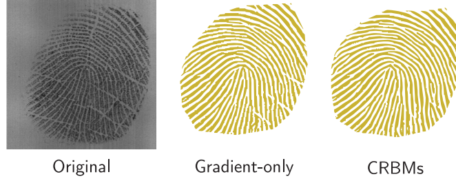
Figure 3.8 A comparison between Gradient-only orientation field estimation and the proposed approach. The proposed approach is more successful in removing creases, and doesn't distort the rest of the orientation field estimated by the gradient-based method.
