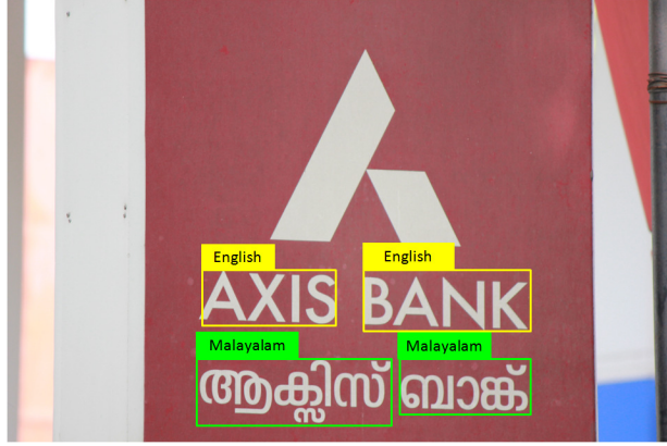
Figure 3.7 An example result of End-to-end script identification of our method. We localize the text boxes in images using method using [33] and [1]. Then we apply our method to find the inherent script in the text boxes.
