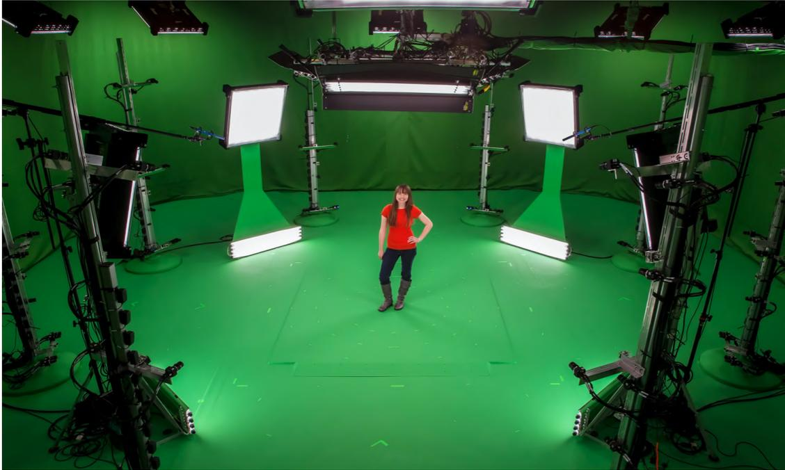
Figure 2.2: An image of a typical multi-view capture setup [22] in a studio with a central stage surrounded by RGB and IR cameras, green screen and static IR laser light sources.
