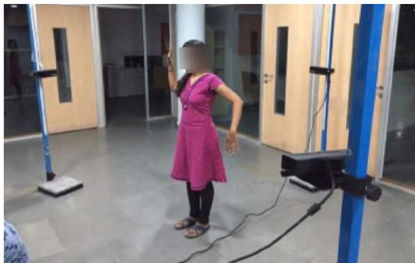
Figure 3.6: **Setup of our 5-Kinect 3D Motion Capture System.**
